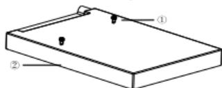
3. Slide the screws in the holes on the chassis bottom from A to B as illustrated and then tighten. Tighten two other screws to fasten the hard disk.
