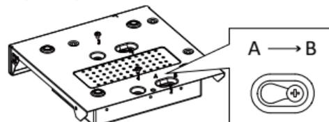
4. Put the cover back in place and tighten the screws.
