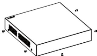
2. Insert the screws (e.g., ①) into the disk (②) and tighten halfway.
